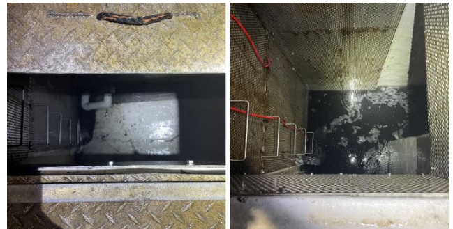
Left: empty hold Right: hold w/ small amount of standing "stick water"
