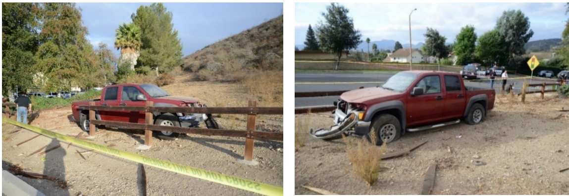
Photograph depicting damage to the front grill/bumper area of Johnson's truck as a result of colliding into the tree and wooden fence. The left front, left rear, and right rear tires were flat.
